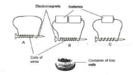
Which of the following options shows the most likely observation Dayne would have made for electromagnet A and B?
