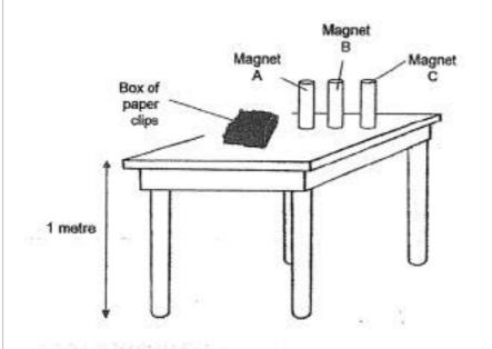
He placed each magnet into a box of paper clips and recorded the number of paper clips attracted to it. He then dropped each of the magnets 5 times from a table of height 1 metre. After which, he tested the number of paperclips attracted by each magnet again and recorded the results in the table below.
